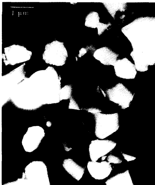
FIG. 1. SEM image showing morphology of the fresh \text{Bi}_2\text{Mo}_2\text{O}_9 catalyst.
